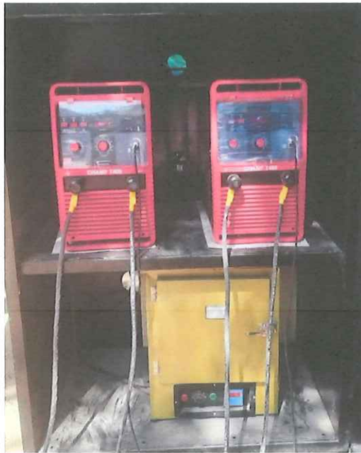
Typical Arrangement of Welding Machine at Site.
