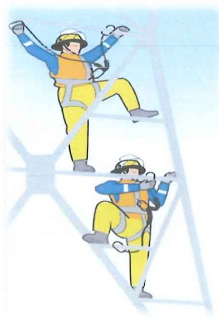
Typical schematic of lead climbing with use of double lanyard fall arrest system technique in RF tower.
